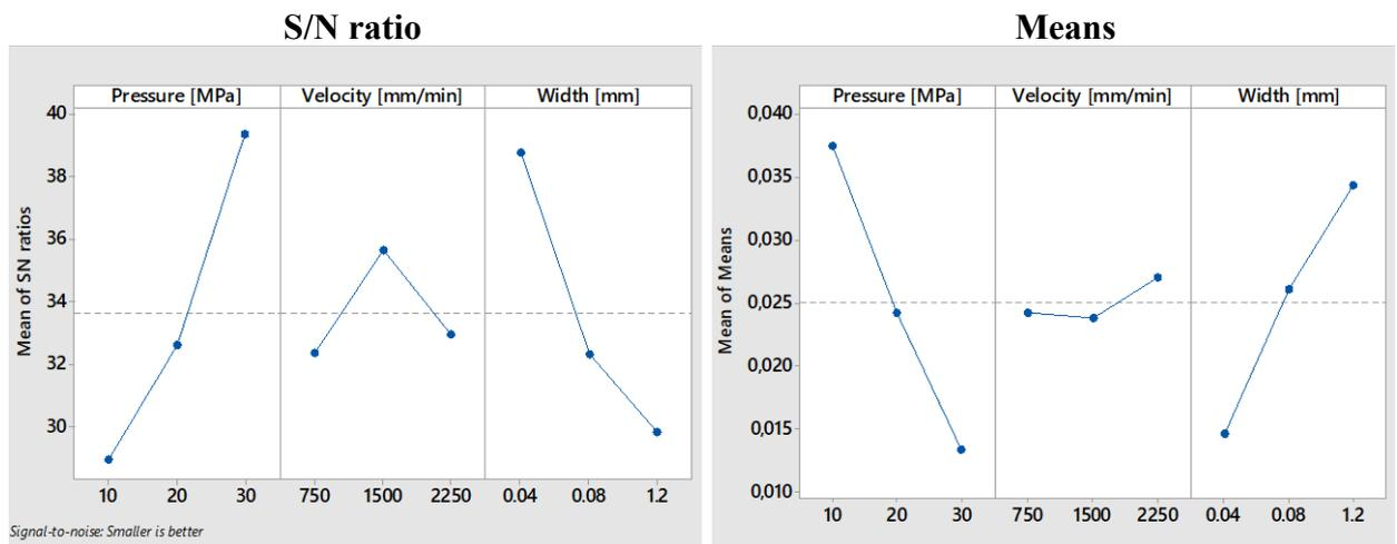
Figure 4: Main effect plots for the S/N ratio and means of Sdr parameter
