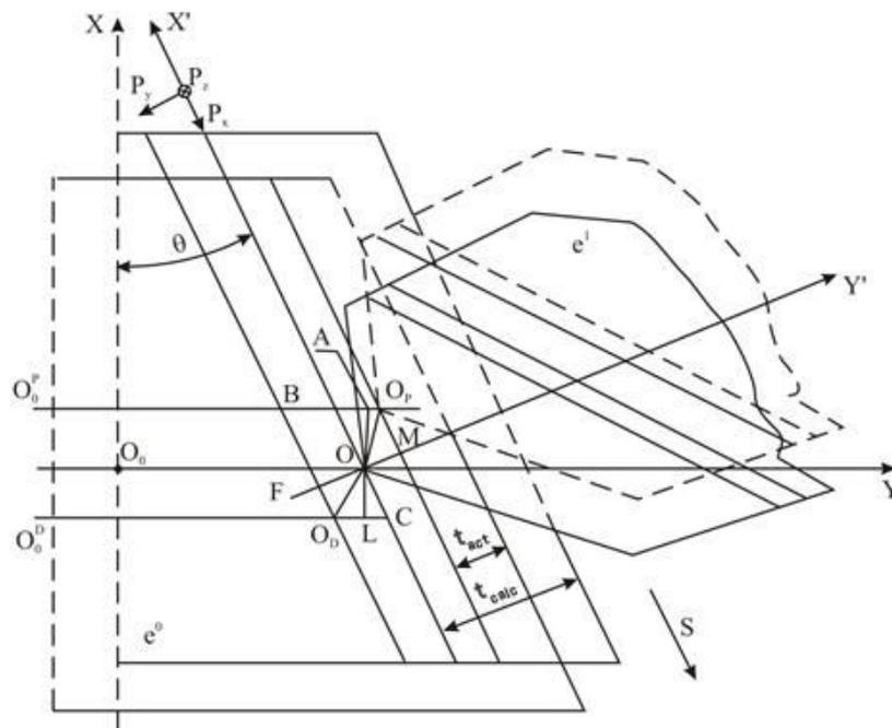
**Figure 1:** Spatial computational scheme of elastic displacements in technological subsystems during single-tool machining with a rotating carriage [11]
