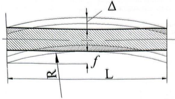
**Figure 2:** Determining the limit value of bending
