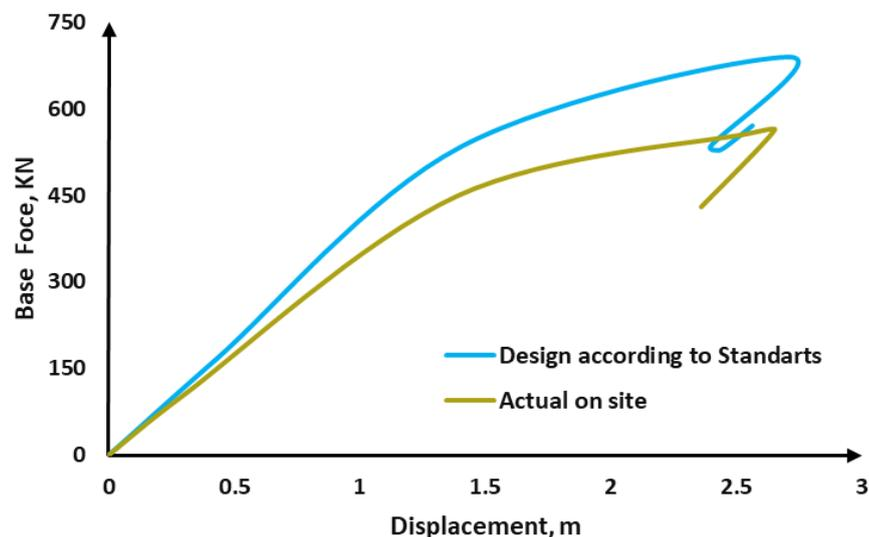
Figure 9. Pushover curve of the overall steel structure
