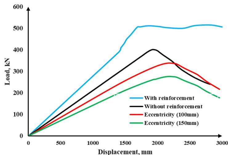
Figure 6. Load displacement curve of column
