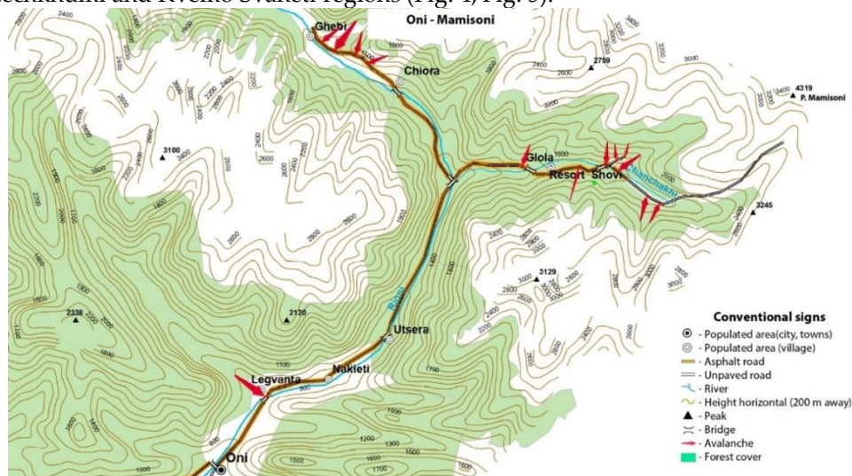
Figure 4: Avalanche hazard map of Oni-Mamison section of the highway of Racha-Lechkhumi and Kvemo Svaneti region
