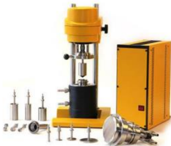
Figure 1. The general view of the rotational rheometer "Rheotest RN 4.1".
