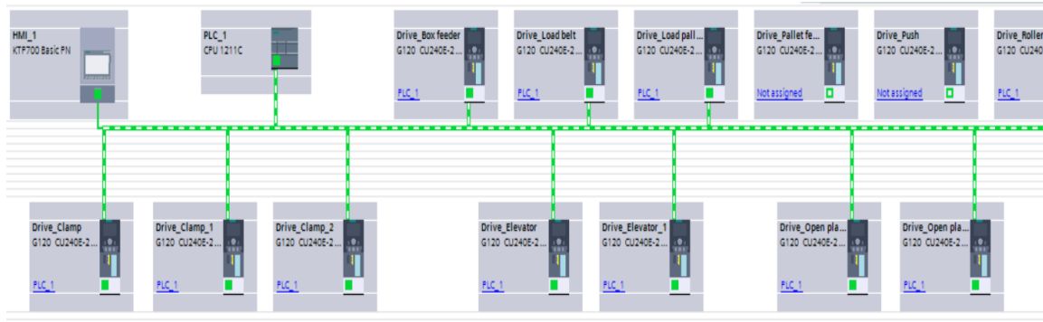
Figure 3: Link with the controller
