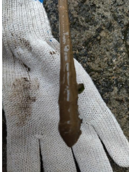
Figure 2: Waterlogged soils on the extracted probe
