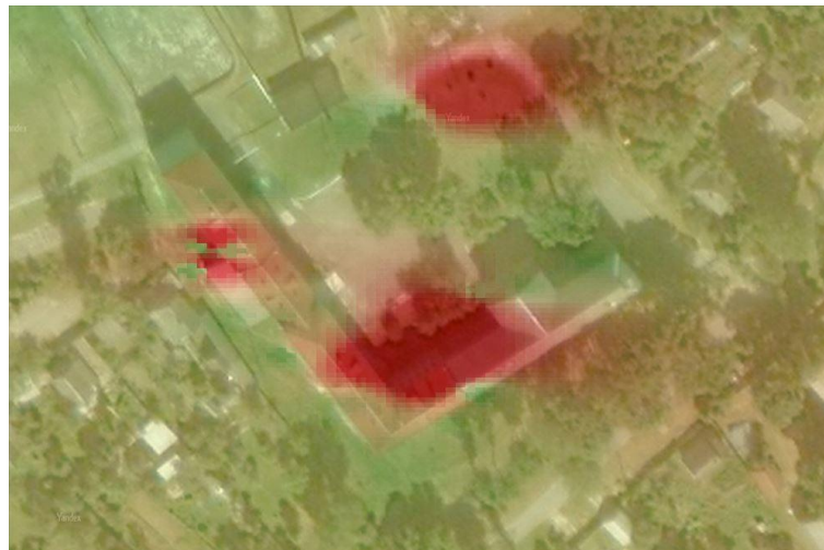
Figure 4: High karst hazard zones (red) at the school construction site, obtained from the results of processing DGM
