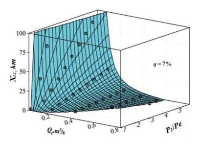
**Figure 2:** Dependence of the distance to the leak point in subsea pipelines on the flowrate and pressure ratio (q=7%)
