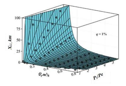
**Figure 1:** Dependence of the distance to the leak point in subsea pipelines on the flowrate and pressure ratio (q=1%)
