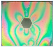
(y) n6 O140 A300 P1000 **Figure 10:** Images of test specimen captured during photoelastic experimental work (n = 6)
