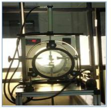
(*a*) photoelastic apparatus
