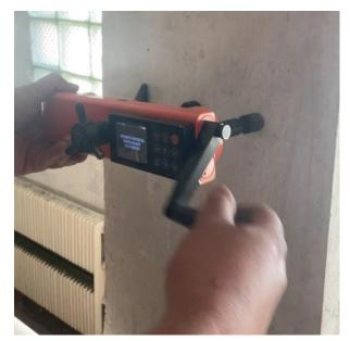
Picture 1: Shear test method using ONIX-1.OS
