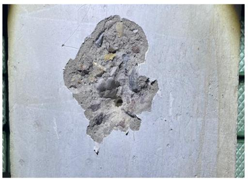
Picture 4: Breaking out of concrete during a shear test
