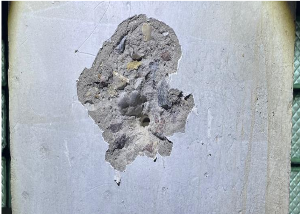
Picture 4: Breaking out of concrete during a shear test
