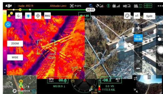
Figure 3: Drones with thermal imaging from DJI Monitoring of insulation and thermal conditions of equipment
