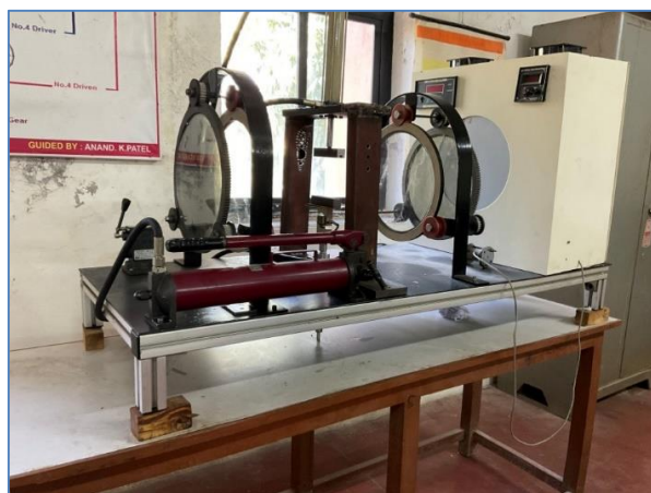
Figure 3: Photo elasticity experimental apparatus
