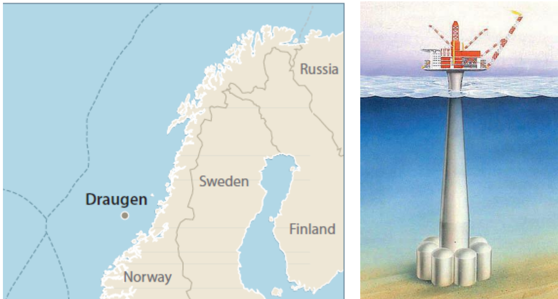
Figure 3. Location plan and general overview of Draugen Monopile Condeep platform [17].
