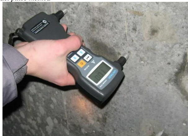
Picture 8: Ultrasonic method
