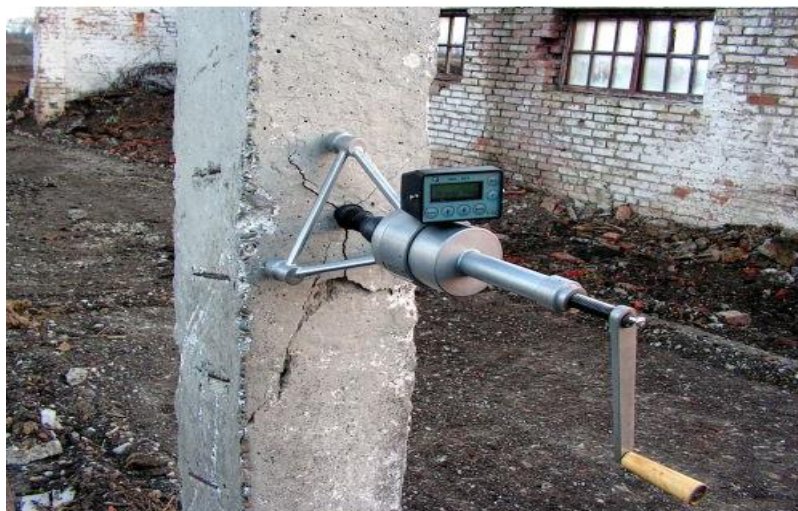
Picture 1: Shear test method
