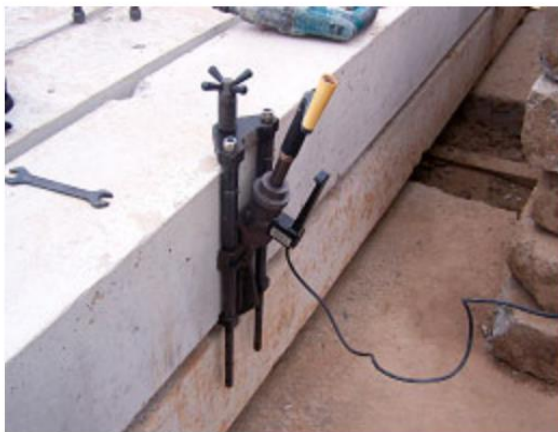
Picture 4: Edge chipping method
