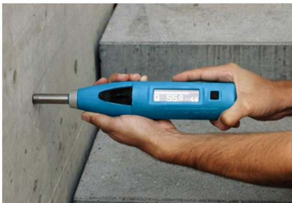
Picture 6: Impact pulse method
