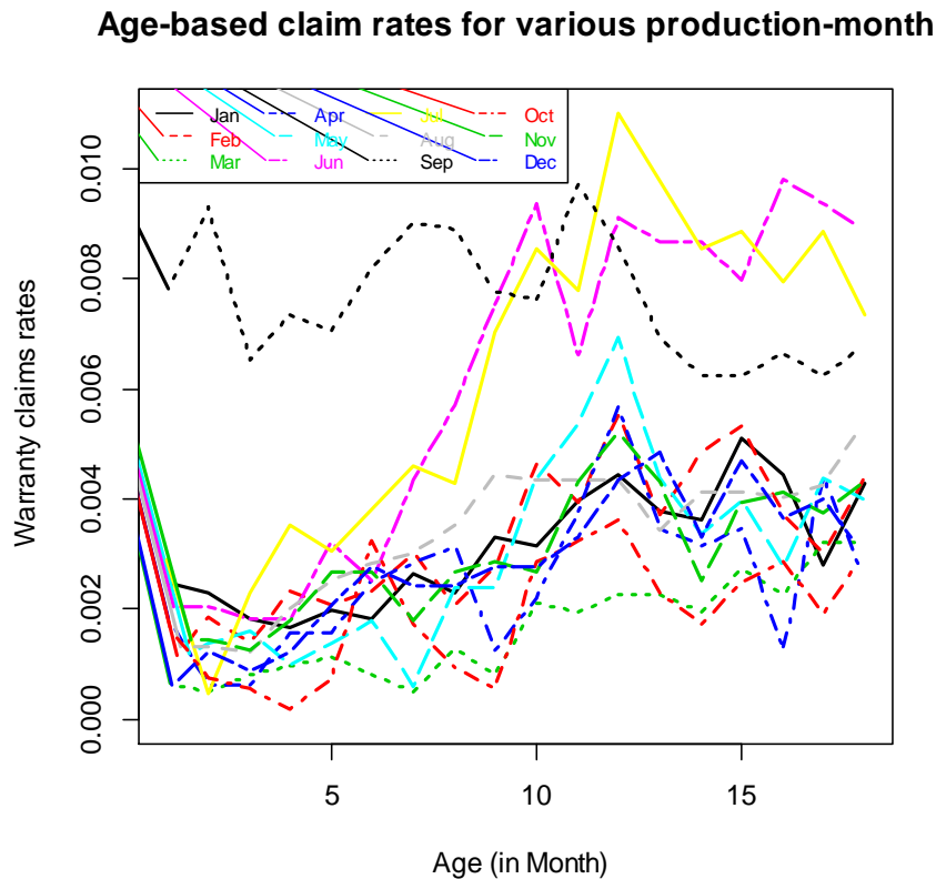
Figure 7: Age-based warranty claim rates for different months of production (Jan. to Dec.)
